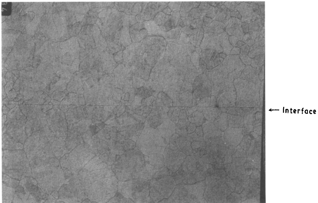
Figure 2 Cross-section of Be-Cu couple diffusion-bonded in a vacuum at 1475°F (802°C) for 2 h showing the bond interface (100 ×).
